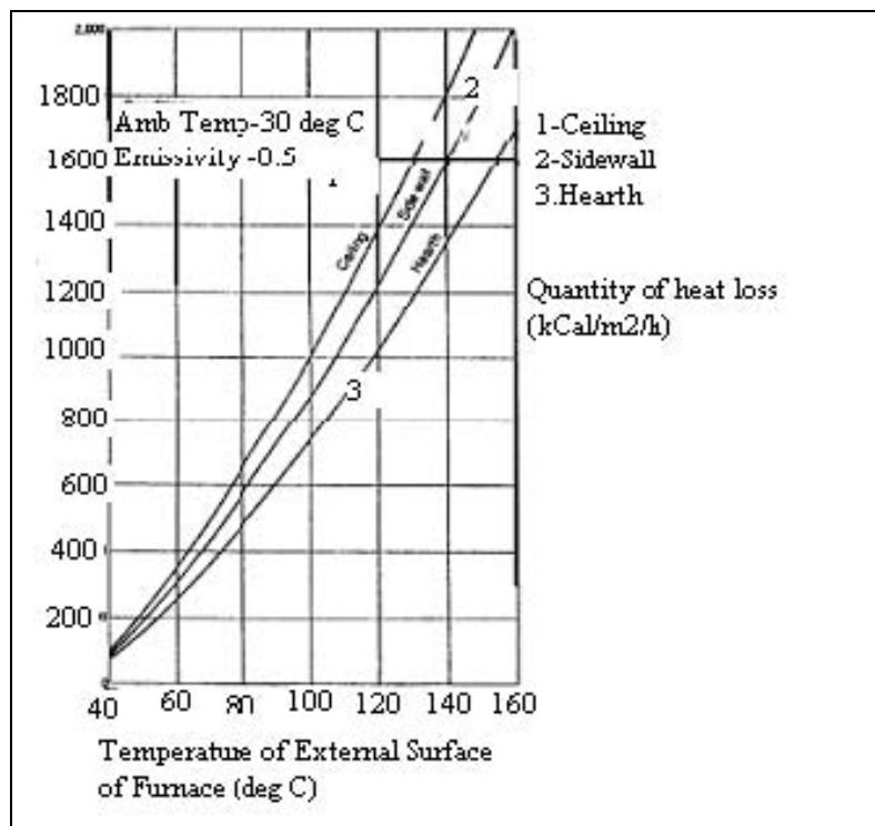
**Figure 15. Relationship between Surface Temperature and Quantity of Heat Loss (BEE, 2005)**
