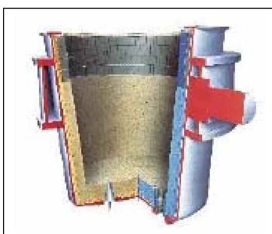
**Figure 9. A Monolithic Lining for Ladle**
