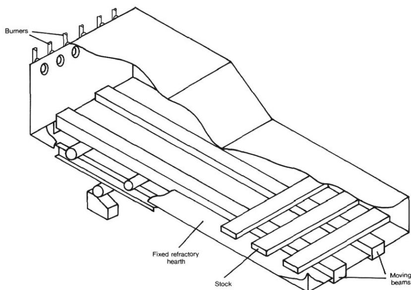
**Figure 6. Walking Hearth Furnace** (The Carbon Trust, 1993)
