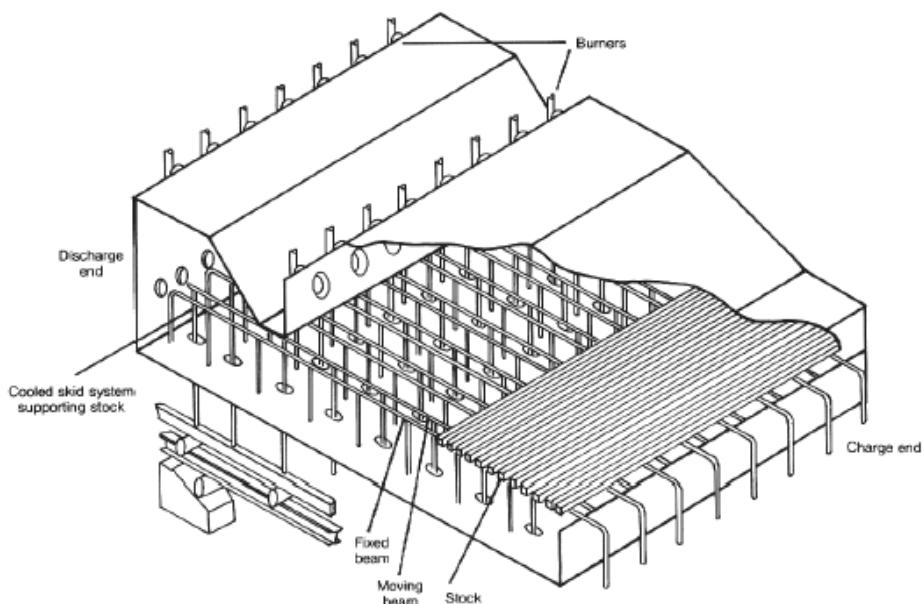
**Figure 5. Walking Beam Furnace** (The Carbon Trust 1993)
