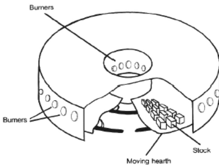
**Figure 8. Rotary Hearth Furnace** (The Carbon Trust, 1993)
