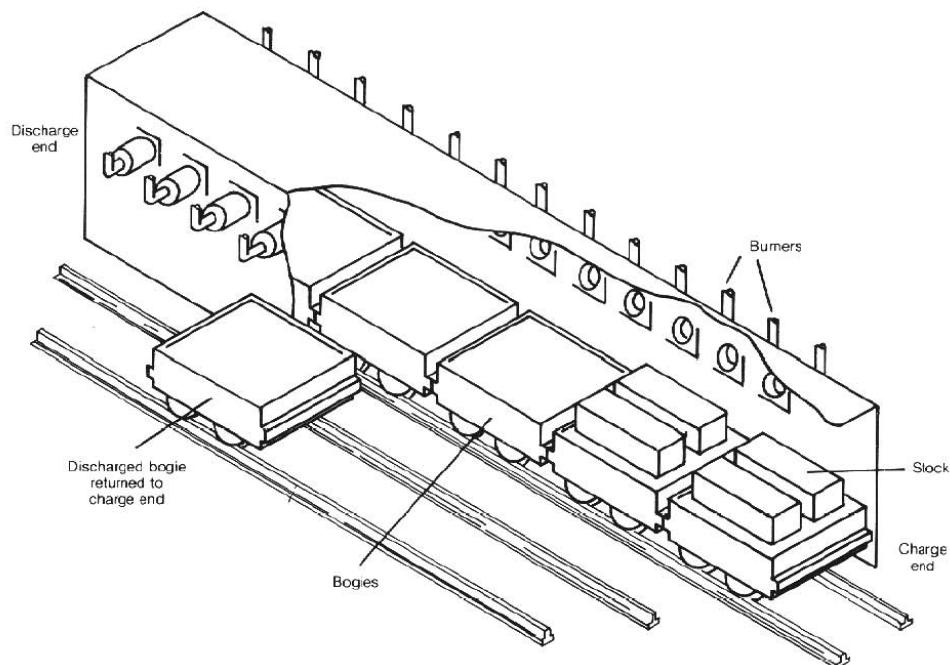
**Figure 7. Continuous Re-circulating Bogie Furnace** (The Carbon Trust, 1993)
