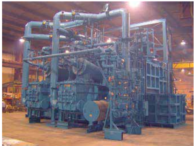
Figure 5 — Lindberg/MPH reverberatory with regenerative combustion.
