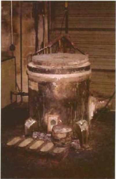
Figure 3: Typical of an older gas fired furnace of 5-to 10 percent energy efficient variety still in use in many plants today.
