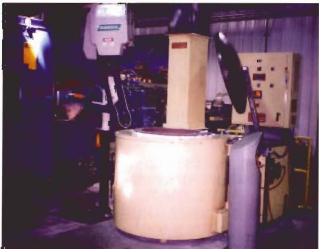
Figure 2: Energy efficient, robot ready gas fired furnaces are available with features such as fully automatic UI, Listed Controls, insulated pneumatic furnace lids, flue stacks to reduce noise and raise heat and fumes above the operators head.
