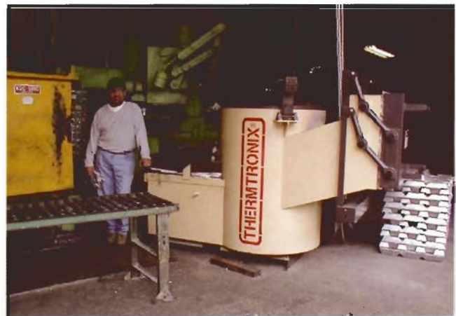
Figure 5: Energy efficient Non-Crucible furnace melting and holding aluminum at the die cast machine
